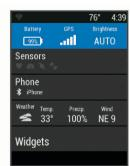
The status page appears. A flashing icon means the device is searching for a signal. A solid icon means the signal was found or the sensor is connected.
